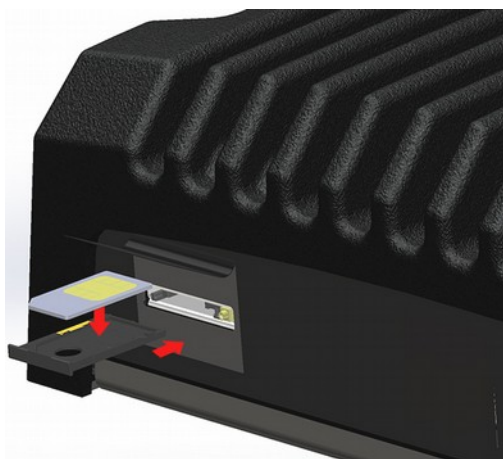
Fig. 4. Inserting a SIM card in to the MCC15 computer unit.
