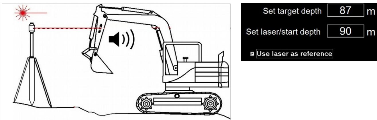
Fig. 28. Moving the receiver to the laser beam (height reference is fed in to the system)
